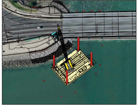
Stage 1: East abutment piling - this diagram shows the jack-up barge with demarcation buoys (red circles). The incoming, outgoing, and reserve channels will be open.
