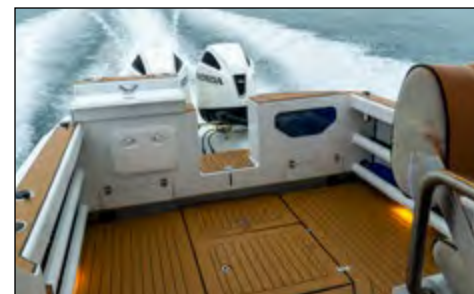
Two 200hp Hondas had the test boat hitting 42 knots at the maximum 5900rpm.
