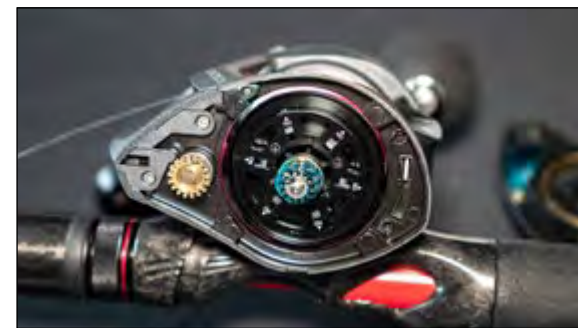
Adjusting the cast control - in this case housed behind the left side plate - will give you more control over the reel.
